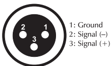
DMX-output XLR mounting-socket:
