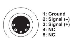
DMX-output XLR mounting-socket:
