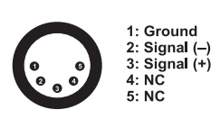
DMX-input XLR mounting-plug:
