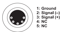
DMX-output XLR mounting-socket:
