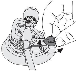
Fig. 8: Adjusting anti-skating
