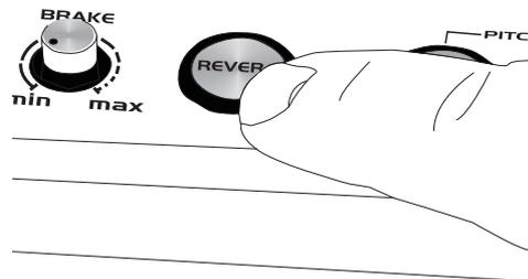
With the button **[REVERSE]** you can switch over the sense of rotation. For this purpose shortly press the button. With the reverse run switched on, the button lights up.
