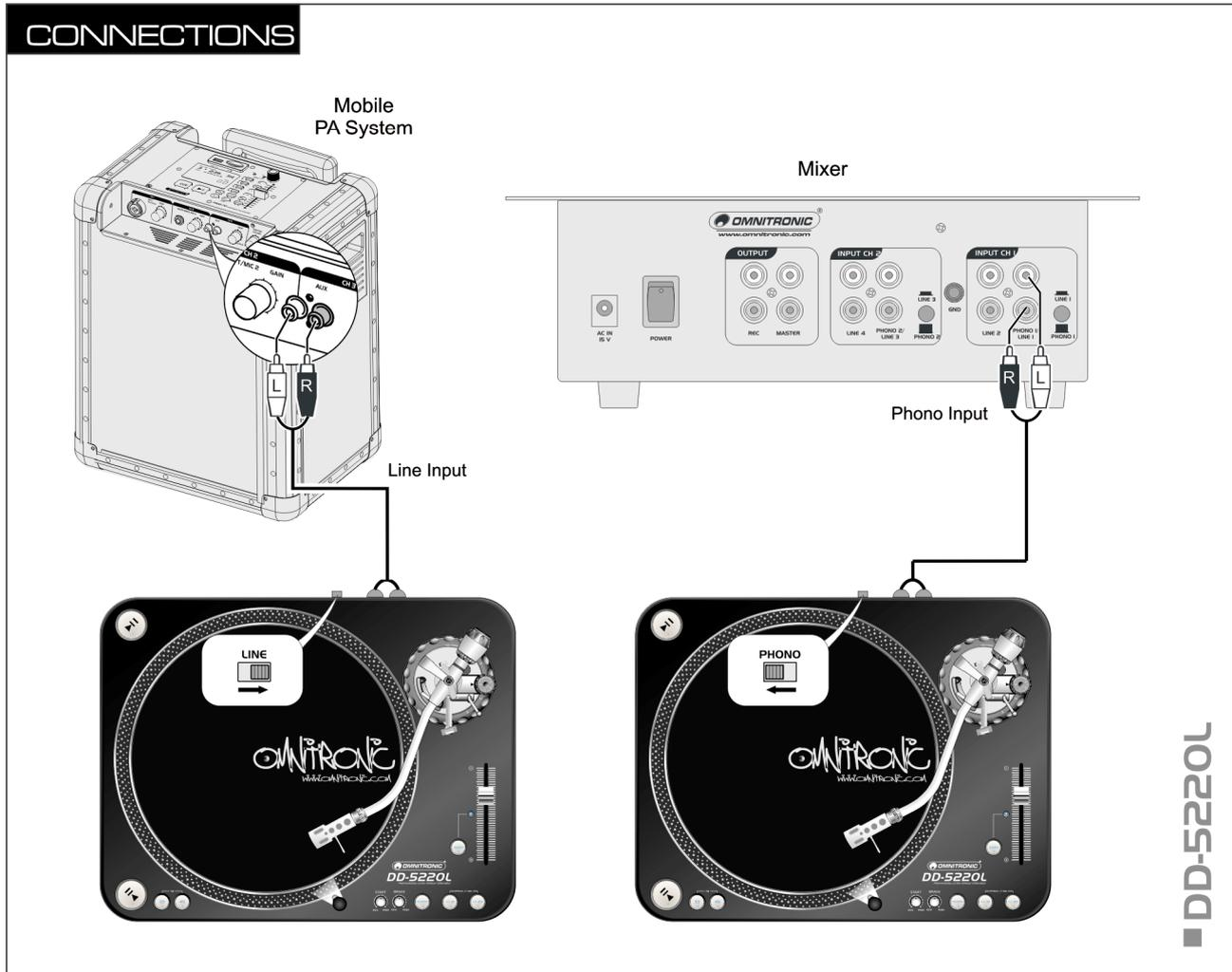
Prior to connecting or changing existing connections switch off the turntable.
