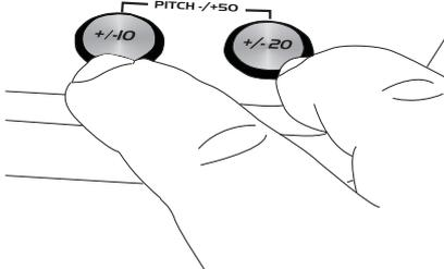
To switch to  $\pm 50\%$  press the buttons **[+/- 10]** and **[+/- 20]** simultaneously.
