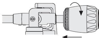
Fig. 5: Mounting the counterweight
