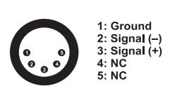
If you are using controllers with this occupation, you can connect the DMX output of the controller directly with the DMX input of the first device in the DMX chain. If you wish to connect DMX controllers with other XLR outputs, you need to use adapter cables.
