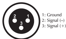
DMX-output XLR mounting-socket:
