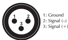
DMX-input XLR mounting-plug:
