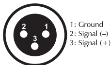
DMX-output XLR mounting-socket:
