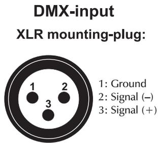
If you are using controllers with this occupation, you can connect the DMX output of the controller directly with the DMX input of the first device in the DMX chain. If you wish to connect DMX controllers with other XLR outputs, you need to use adapter cables.
