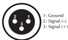
DMX-output XLR mounting-socket:
