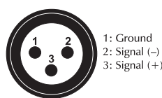
DMX-input XLR mounting-plug:
