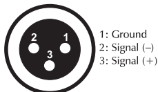
DMX-output XLR mounting-socket:
