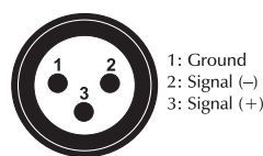
DMX-input XLR mounting-plug:
