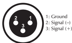
DMX-output XLR mounting-socket:
