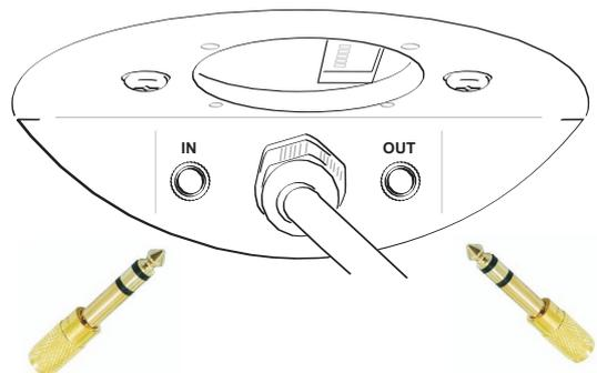
Connection between devices is carried out via special connection cables having stereo jack plugs, included in delivery.
