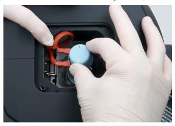
4. Gently remove (2) Wires connected to spade terminals on lamp. (See below)
