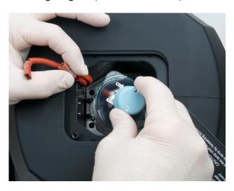
7. Gently attach (2) Wires to spade terminals on the base of the lamp. (See below)
