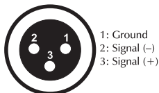
DMX-output XLR mounting-socket:
