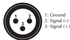
DMX-input XLR mounting-plug:
