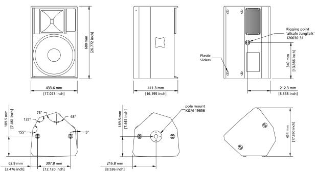
Further information and data like specifications, manuals, technical drawings as DWG, DXF and PDF files as well as data files for acoustic simulations with Ease and Ulysses are available on our web site www.kling-freitag.de
